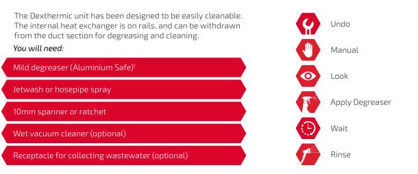
It's essential to use cleaning chemicals and degreasers that are safe for aluminium surfaces and to follow the manufacturers' recommendations and mixing ratios.<sup>1</sup>
